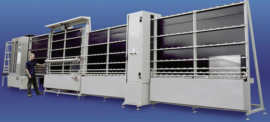
The Atlantic computerised line is designed to streamline production of insulated glass units. The line speeds up assembly times using a primary seal or self adhesive tape on the spacer bar and eliminates the need to touch the glass after washing. Standard units are produced with the line in automatic mode, shapes in semi-automatic, and wash only mode if the assembly line is not required.
